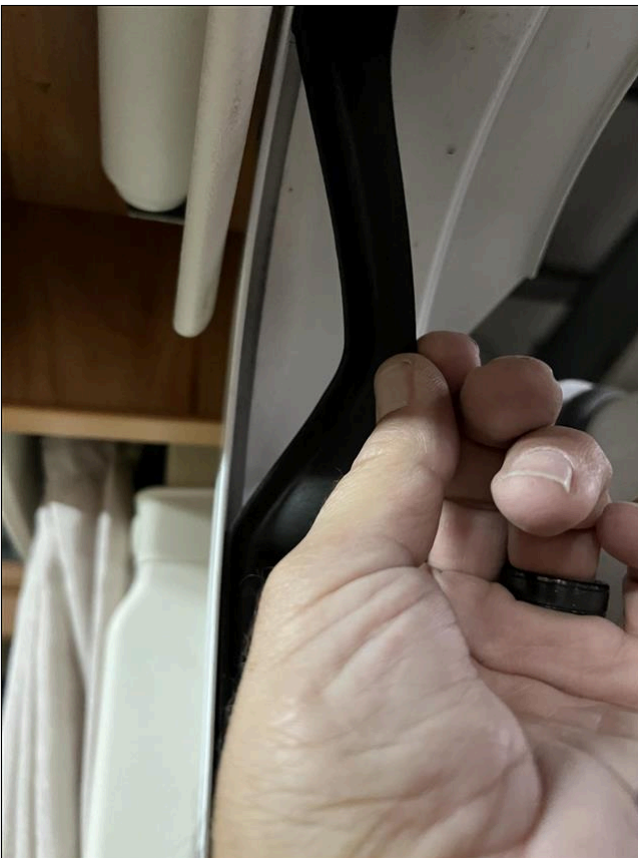
(2) Upper left and right seal of the door frame is coming detached.
