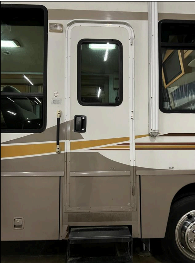
(2) Upper left and right seal of the door frame is coming detached.
