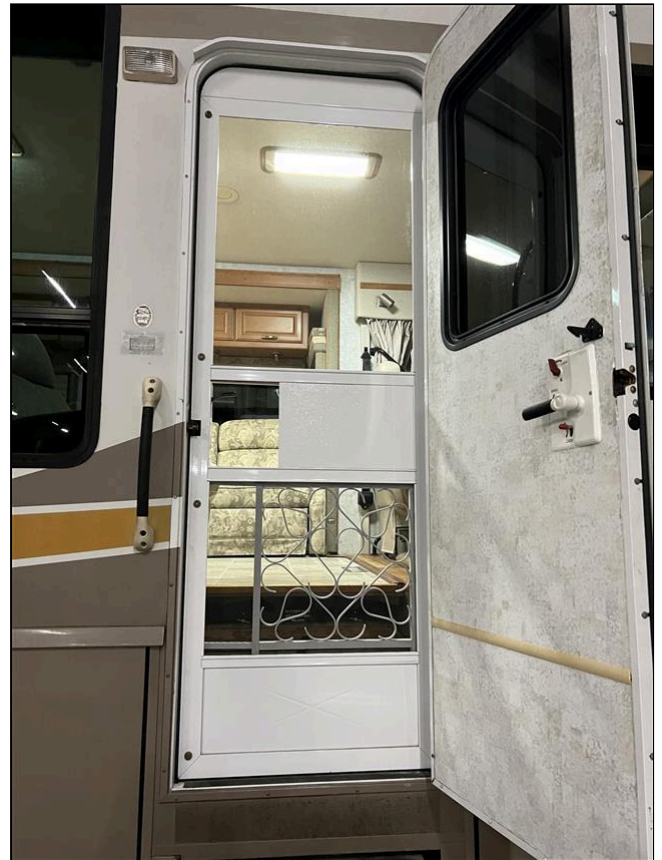
(2) Upper left and right seal of the door frame is coming detached.
