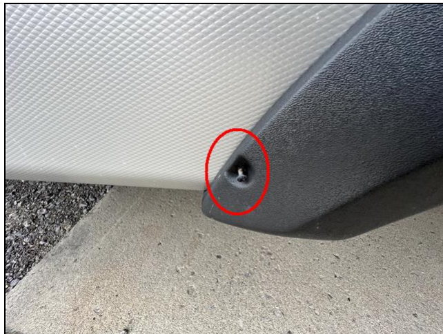
(2) Dents and a screw in the lower fender wall.
